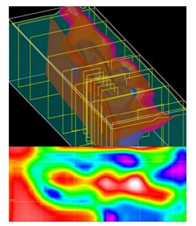
Figure 1, upper: Pilbara model of BIF (vertically exaggerated 3:1) used to capture geological uncertainty in grade-tonnage estimates, using a potential field method of interpolating implicit 3D surfaces. Lower: Computed forward response of the gravity gradient Gzz from 3D geology. Units are Eotvos.
