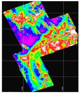
Figure 2: Montezuma gridded tensor data with a phase enhancement derived from rotating each tensor to solve the Eigen system (hence like an AGC filter), histogram equalised. The NE cross-cutting fault and N20W rift bounding fault are clear.
